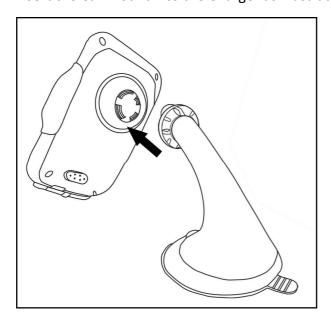
3. Tighten it by turning the Knob clockwise as illustrated below:
