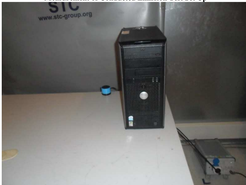
Measurement of Conducted Emission Test Set Up
