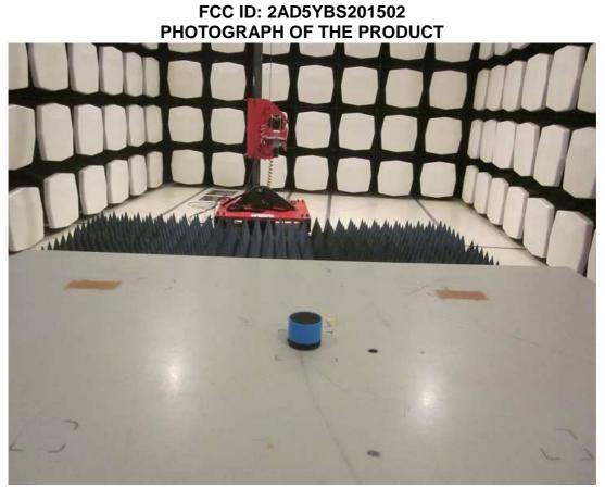
MEASUREMENT OF CONDUCTED EMISSION TEST SET UP
