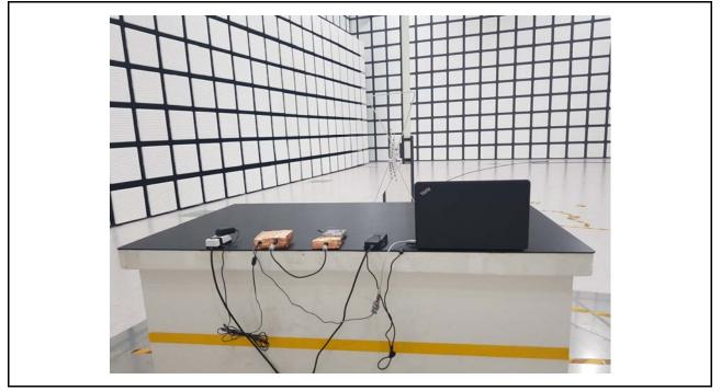
3. Radiated Emission setup photo (above 1 GHz)
