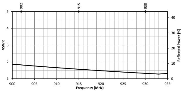
Figure 4. ANT-915-IPW1-RPS Antenna VSWR, Edge Bent
