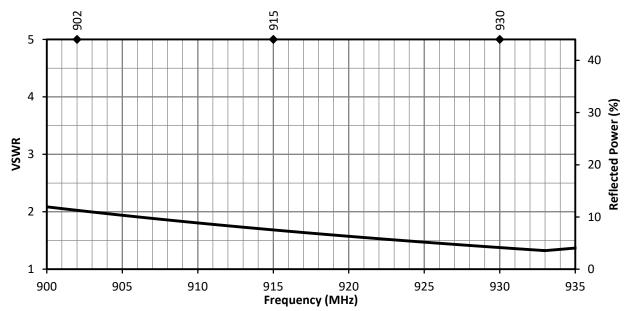
Figure 11. ANT-915-IPW1-RPS Antenna VSWR, Straight
