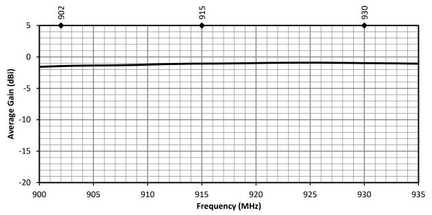
Figure 14. ANT-915-IPW1-RPS Antenna Average Gain, Straight
