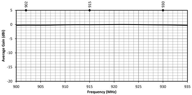
Figure 7. ANT-915-IPW1-RPS Antenna Average Gain, Edge Bent
