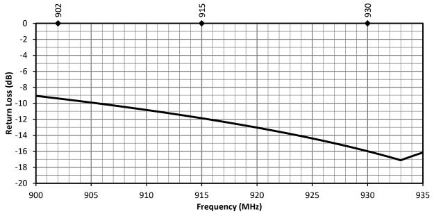
Figure 12. ANT-915-IPW1-RPS Antenna Return Loss, Straight
