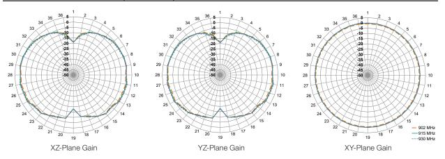
Figure 16. Radiation Patterns for ANT-915-IPW1-RPS, Straight
