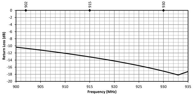
Figure 5. ANT-915-IPW1-RPS Antenna Return Loss, Edge Bent
