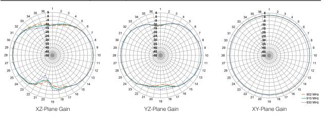
Figure 9. Radiation Patterns for ANT-915-IPW1-RPS, Edge Bent
