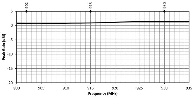
Figure 13. ANT-915-IPW1-RPS Antenna Peak Gain, Straight
