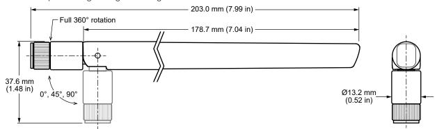
Figure 1. ANT-915-IPW1-RPS Antenna Dimensions
