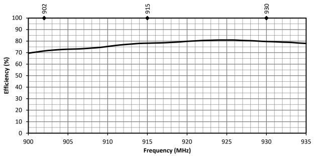
Figure 15. ANT-915-IPW1-RPS Antenna Radiation Efficiency, Straight
