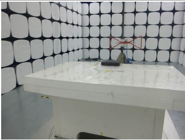
FG9008N Radiated Spurious Emissions Test Setup Below 1GHz
