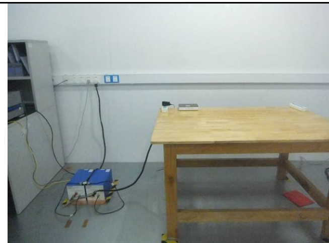
FG9004N Conducted Emissions Test Setup Front View
