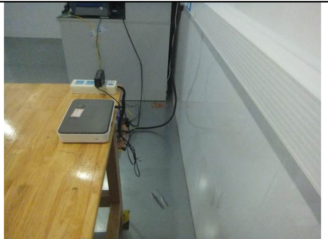
FG9004N Conducted Emissions Test Setup Side View
