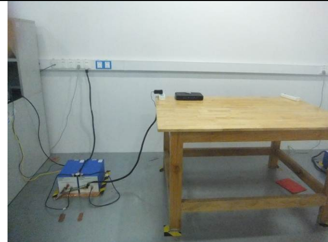
FG9008N Conducted Emissions Test Setup Front View
