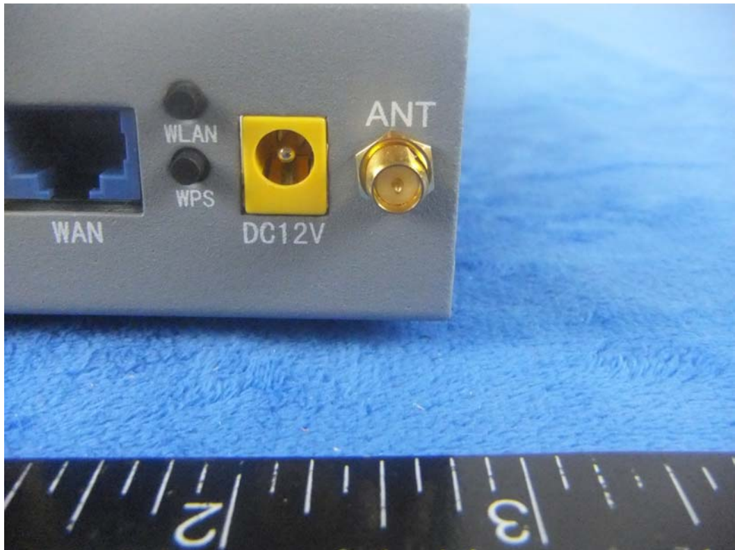
Antenna connector 1 view
