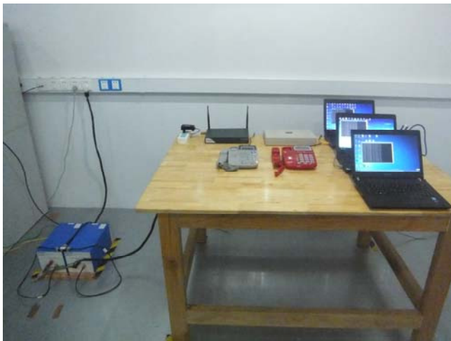
Conducted Emissions Test Setup Front View
