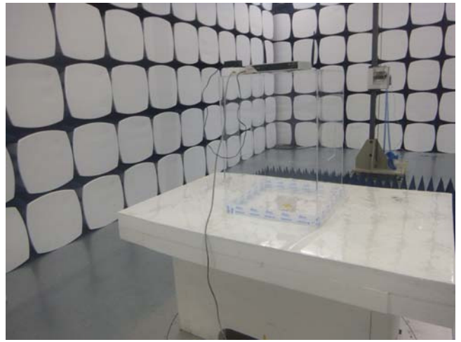
Radiated Spurious Emissions Test Setup Above 1GHz
