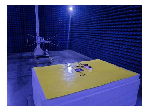
Photo of Radiated Emission Measurement (Below 1G)
