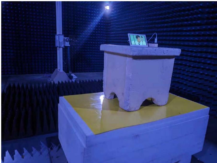
Photo of Radiated Emission Measurement Above 1GHz
