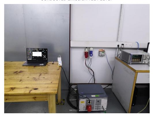
CONDUCTED TEST SETUP
