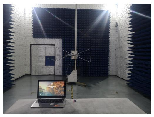
RADIATED EMISSION TEST SETUP ABOVE 1GHZ
