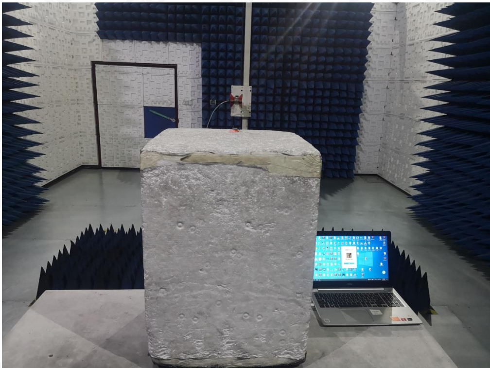
FCC RADIATED EMISSION TEST SETUP ABOVE 1GHZ
