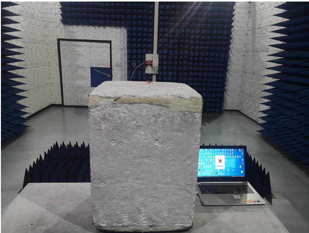
RADIATED EMISSION TEST SETUP ABOVE 1GHZ
