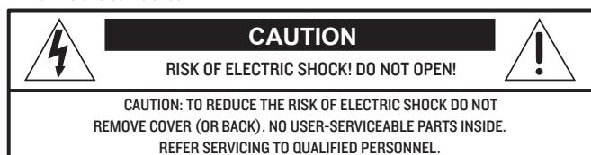
The lightning flash with arrowhead symbol within an equilateral triangle is intended to alert the user to the presence of uninsulated "dangerous voltage" within the product's enclosure, that may be of significant magnitude to constitute a risk of electric shock to persons.
