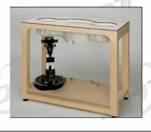
The shell corresponds to the specifications of the Specific Anthropomorphic Mannequin (SAM) phantom defined in IEEE 1528 and IEC 62209-1. It enables the dosimetric evaluation of left and right hand phone usage
