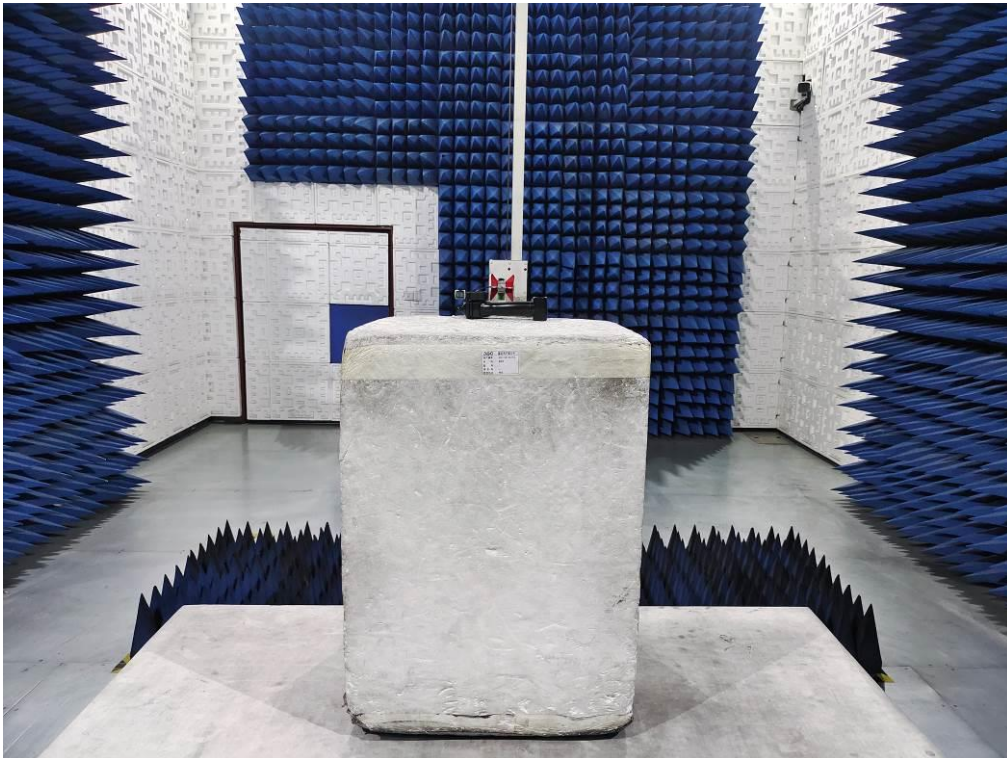
FCC RADIATED EMISSION TEST SETUP ABOVE 1GHZ
