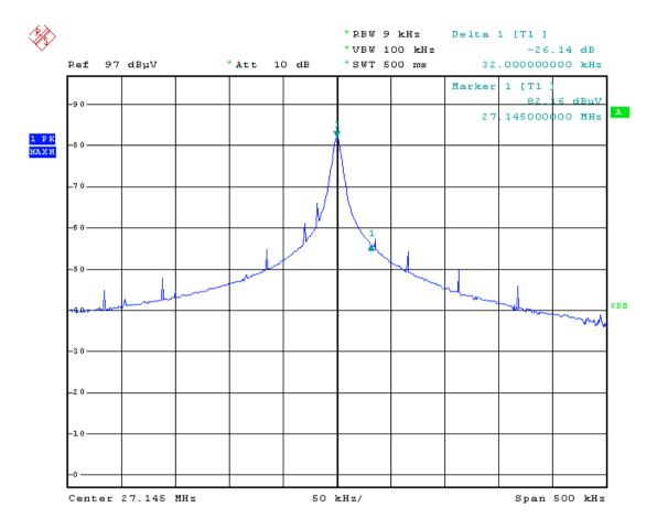
The field strength of any emission within the operation band did not exceed 80 dB(µV/m) for average value or 100 dB( $\mu$ V/m) for peak value.
