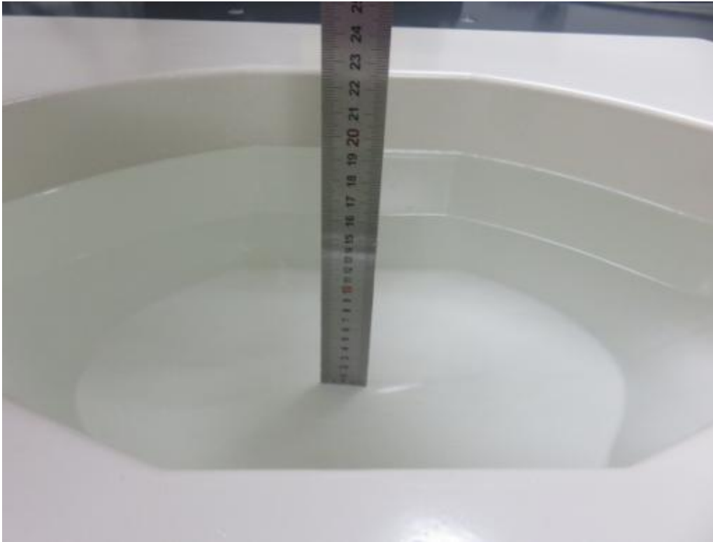
Photograph of the depth in the Body Phantom (5300MHz, 16.1cm depth)
