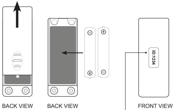
Open the sensor's batteries' compartment to include the provided AAA batteries (x2). Place the batteries as per picture indications. Finally, close the compartment.
