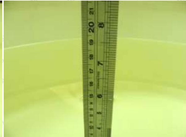
Photo of Liquid Height for Body SAR
