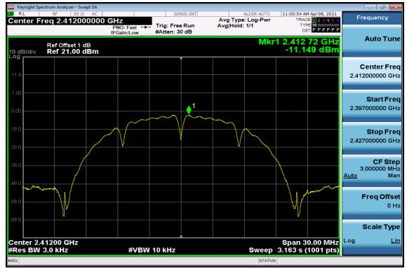
**Power Spectral Density Test Plot (CH-Mid)**
