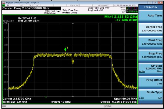
Power Spectral Density Test Plot (CH-High)
