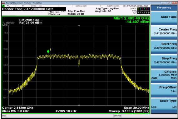
**Power Spectral Density Test Plot (CH-Mid)**
