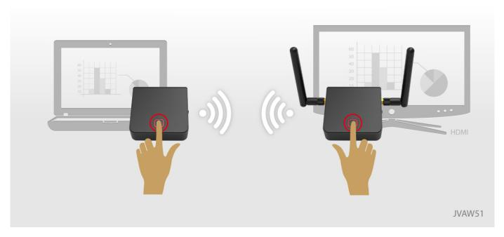
If we connect the paired Rx, but paired Tx didn't connect, we will also see the pic above. Please connect the paired Tx to complete the connection.
