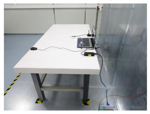
Test Mode: Mode 3 Description: Radiated Emission Test Setup for below 1GHz
