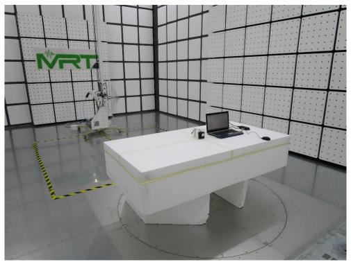
Test Mode: Mode 1 ~ Mode 4 Description: Radiated Emission Test Setup for above 1GHz
