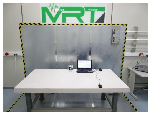
Test Mode 3 Description: Back View of Conducted Emission Test Setup
