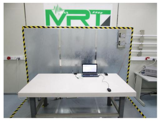
Test Mode 7 Description: Back View of Conducted Emission Test Setup
