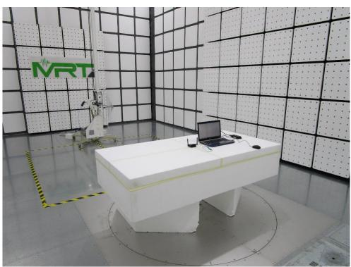
Test Mode: Mode 5 ~ Mode 8 Description: Radiated Emission Test Setup for above 1GHz
