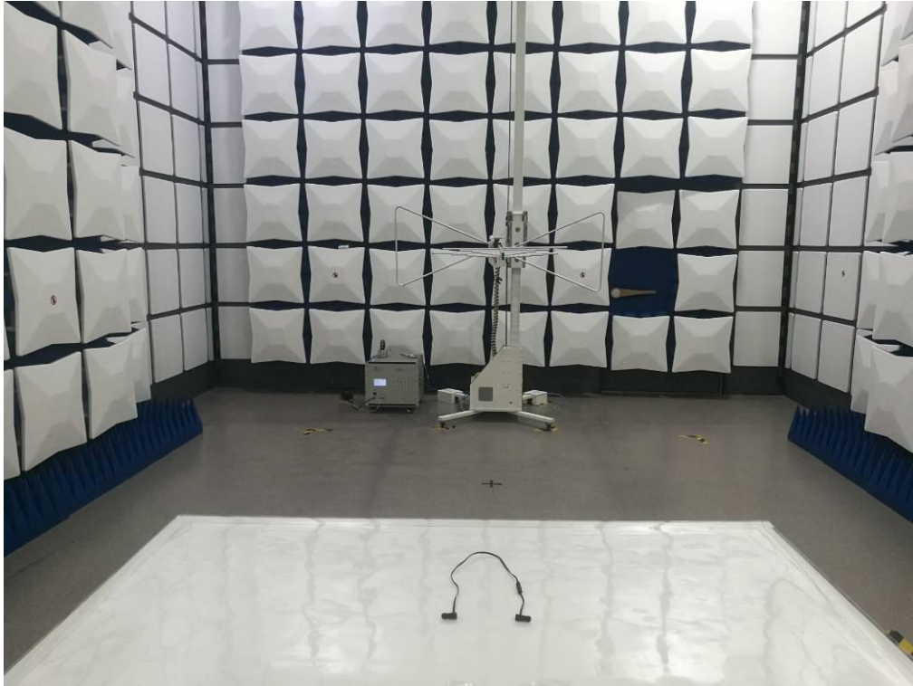
FCC RADIATED EMISSION TEST SETUP
