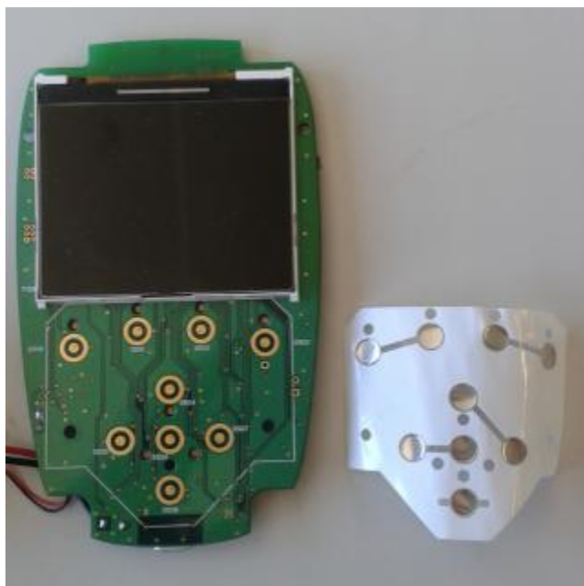
Top side of PCB to show what's underneath the display and keypad, including bottom side of display and keypad
