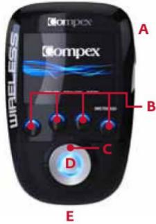
A - On/Off button (press briefly to turn on, hold down for more than 2 sec. to turn off)
