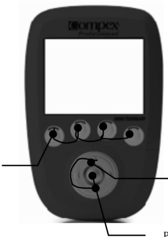
Select the channels on which to act. When a channel is active the LED button emits a strong blue light.
