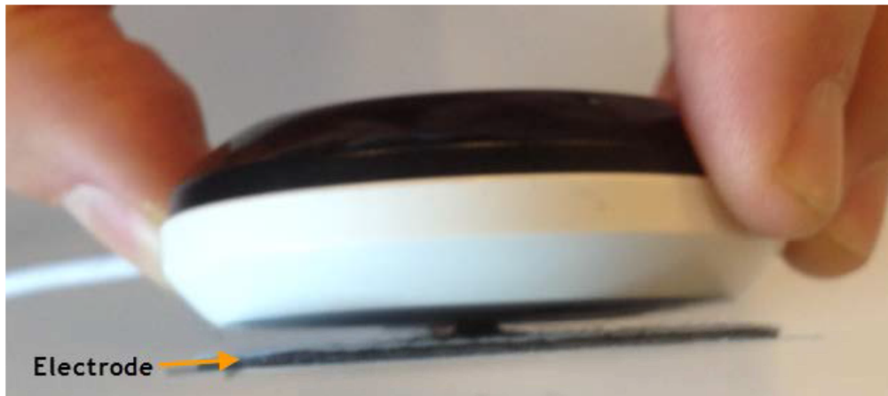
Side view of Module “snapping” into electrode
