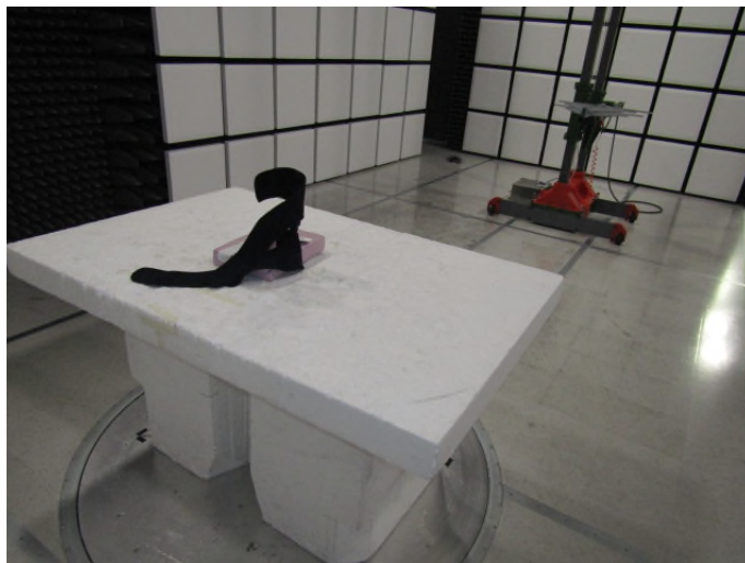
Figure 2: Radiated Emissions – Below 1GHz – Rear View
