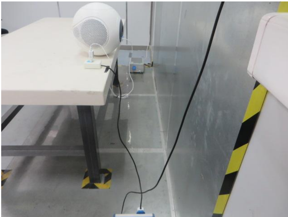
Description: Back View Conducted Emission Test Setup for Power Port ( For Model: MI10 )
