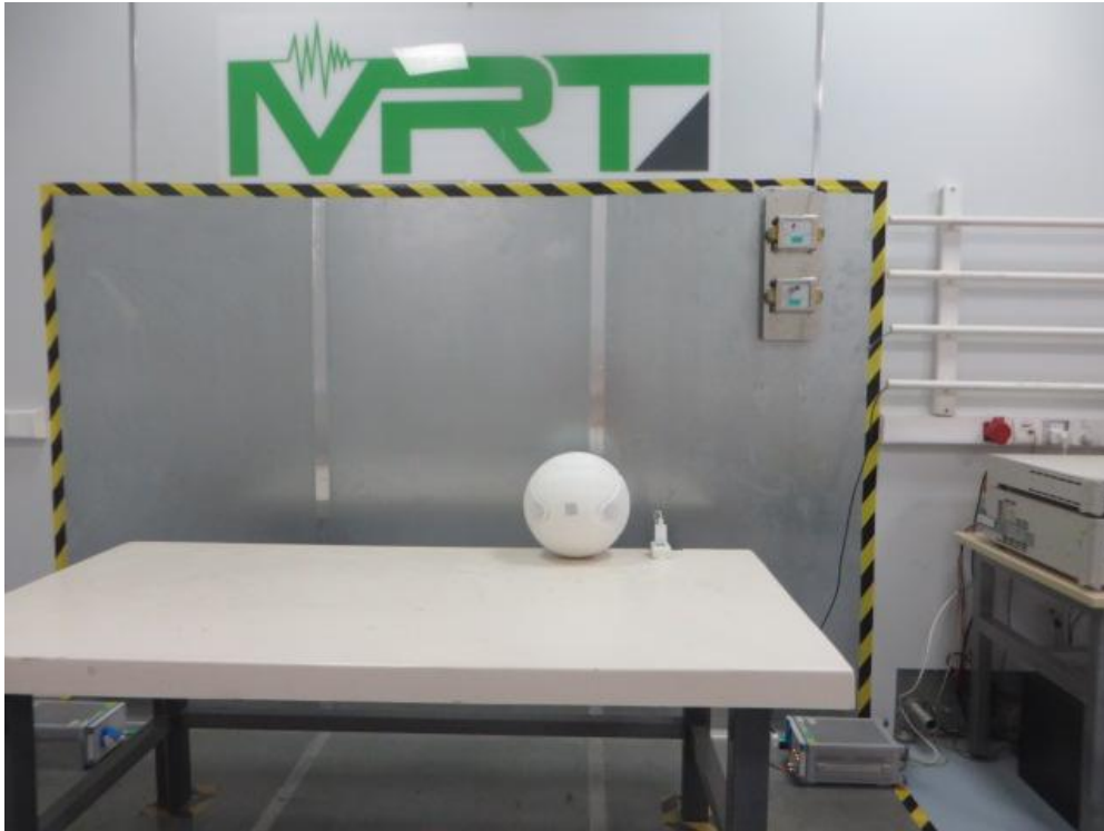
Description: Back View Conducted Emission Test Setup for Power Port ( For Model: MI10 )
