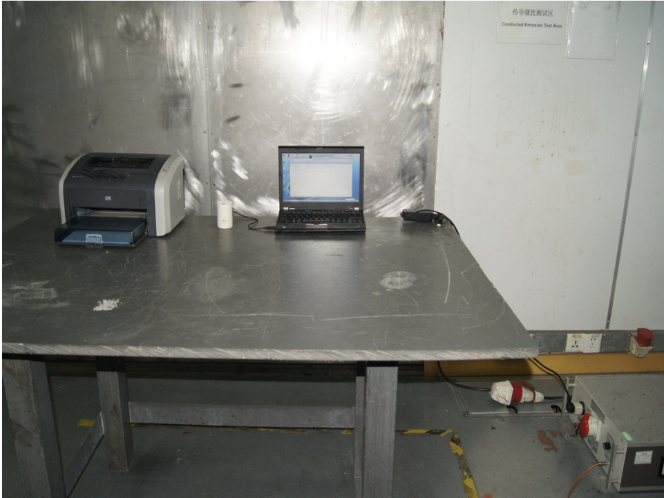
Photograph 6: Set-up for Radiated Emissions, below 1GHz
