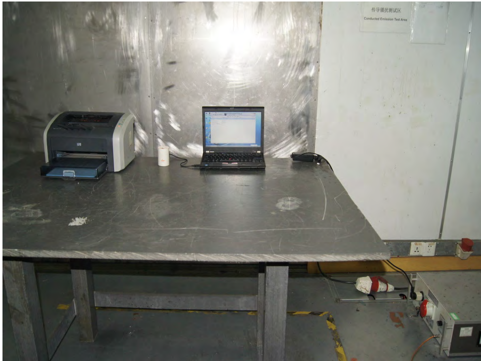
Photograph 6: Set-up for Radiated Emissions, below 1GHz
