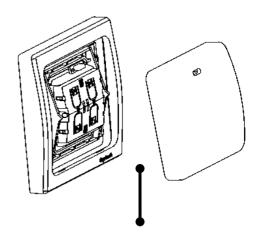
**1.** Separate the key cover from the transmitter.
