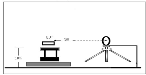
(A) Radiated Emission Test-Up Frequency Below 30MHz
