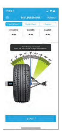
**3.1.2** Allow Sharp Align to calibrate. Once calibrated, a Camber reading will show.
