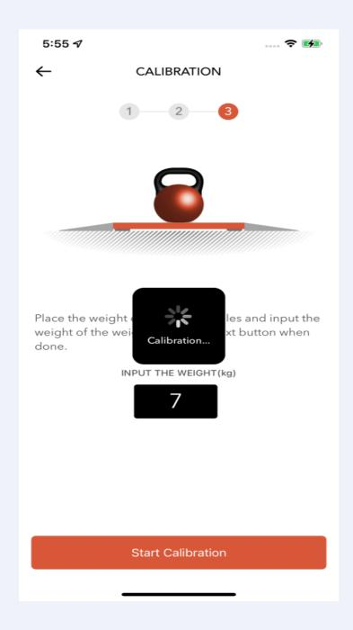
Tap Start Calibration and wait for 10 seconds to complete Step 3.
