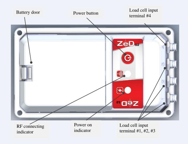
When setting mode, user can using 3-Load cell or 4-Load cell input. If setting for 3-load input, please let terminal #4 open, and load cell connected to #1, #2 and #3.
