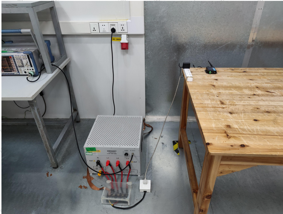
Photo of Conducted Emission Measurement
