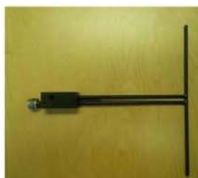
Figure 1 – MVG COMOSAR Validation Dipole
