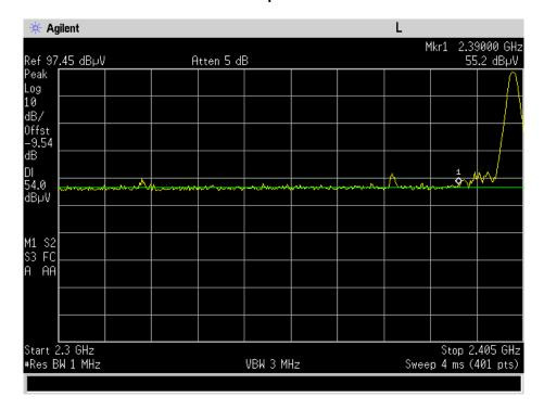
Restricted Band 2300 – 2390 MHz – Avg Tuned Freq = 2402 MHz
