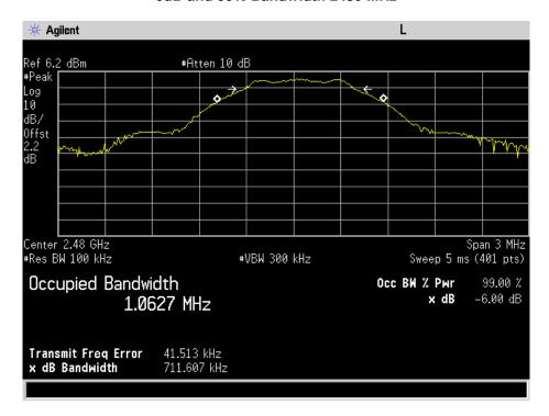
**Transmitter Power Spectral Density (PSD)**
