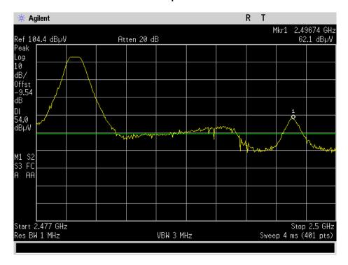
Restricted Band 2483.5 – 2500 MHz – Avg Tuned Freq = 2480 MHz
