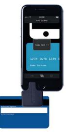
Remove the clear plastic tab from the Stratos Reader and plug into your mobile device.
