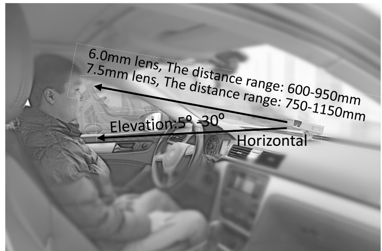
Figure 3 A side view of Installation
