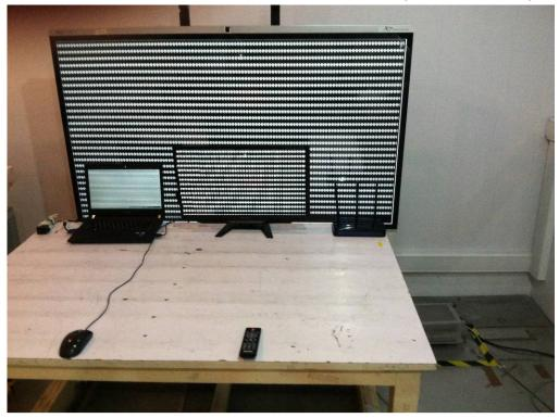
1.2 Radiated Disturbance(30MHz-1GHz) Test Setup
