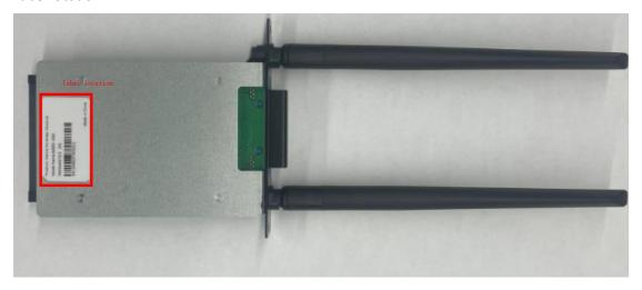
The label is attached to the surface of the shield with a permanent adhesive.
