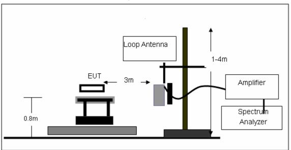
(B) Radiated Emission Test-Up Frequency 30MHz~1GHz
