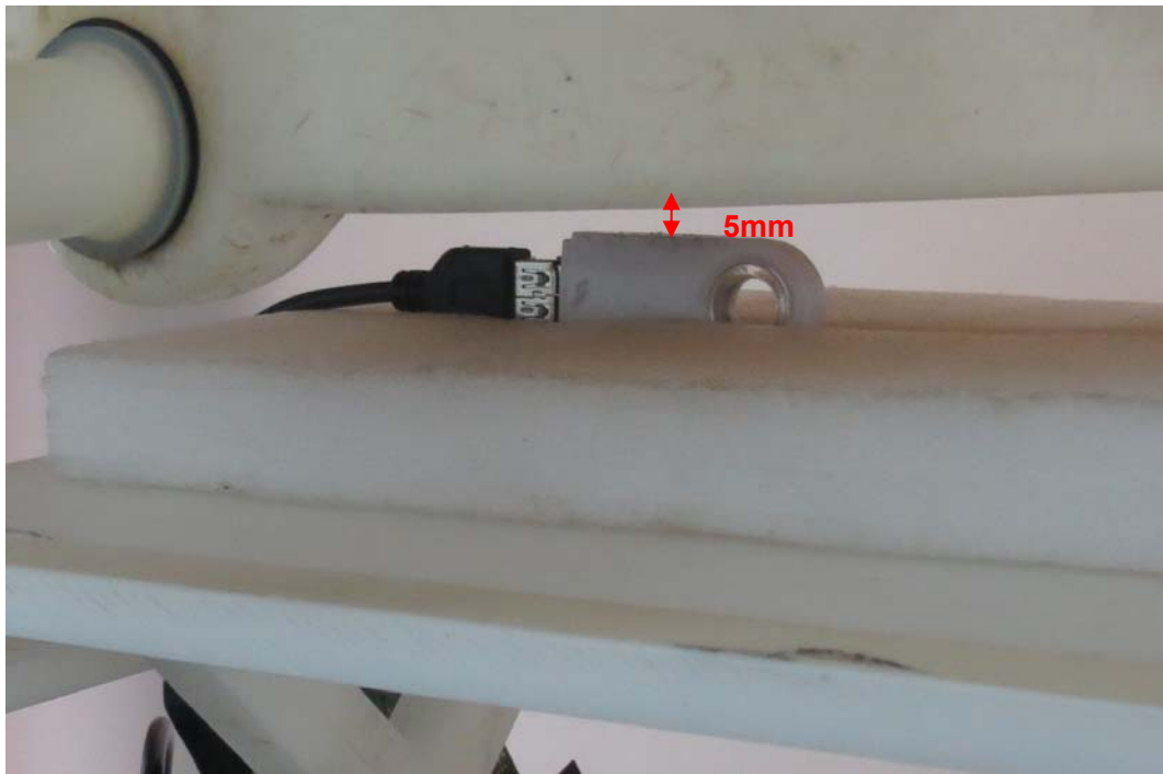
Picture 7: Front Side, the distance from EUT to the bottom of the Phantom is 5mm
