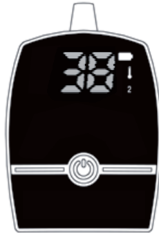
Higher temperature limit is exceeded for BU no. 2
