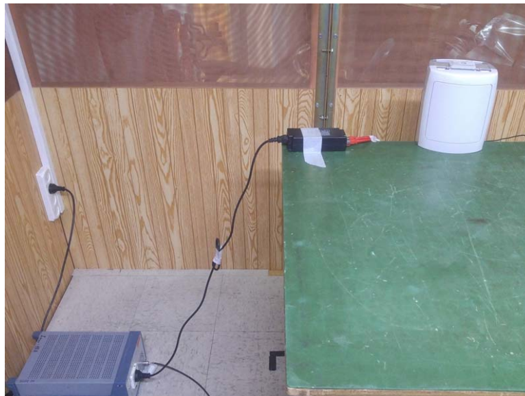
Photograph 8.1.1 Setup for conducted emission measurements
