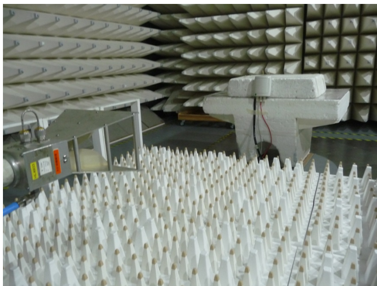
Photograph 8.2.2 Setup for radiated emission measurements in 1-18 GHz
