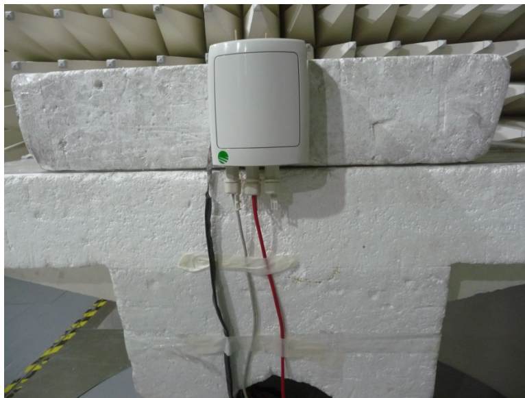
Photograph 8.2.4 Setup for radiated emission measurements, EUT cabling
