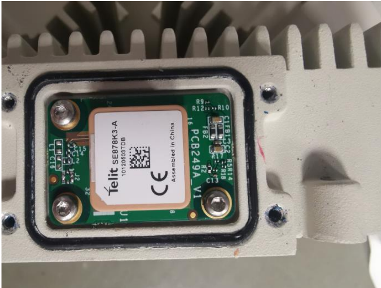
Photograph No.5 MH-N366-CCS-PoE-MWB GPS module
