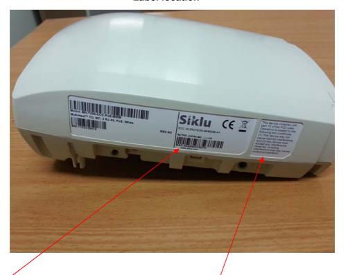
Label with FCC ID:2ACYESK-MH60GE-A1 location, label with the statement according to FCC part 15 §15.19(a)(3)
