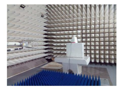
Photograph No.4 Spurious emissions measurement setup in the anechoic chamber in 1-18 GHz
