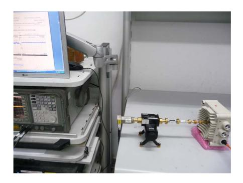
Photograph No.1 Peak output power, OBW, spurious emissions measurement setup
